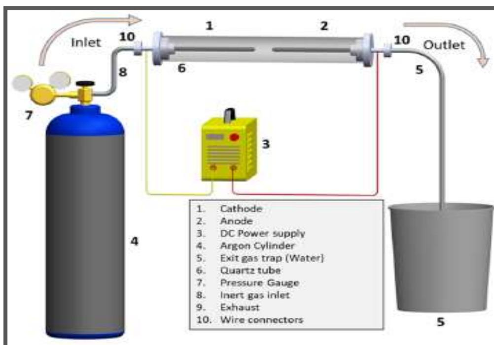
**Fig. 1 Schematics of electric Arc discharge setup under inert gas (Ar) Environment**
