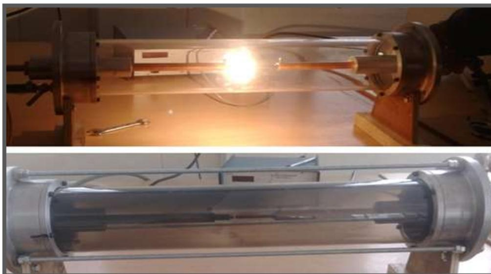
**Fig.5 Intensity of Arching Plasma when arching with Doped graphite rod as anode**
