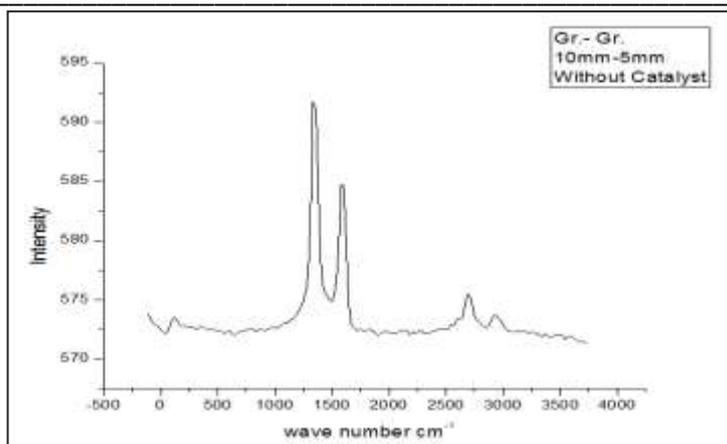
**Fig. 9 Raman analysis of Synthesized Product when pure Graphite used as a Anode**
