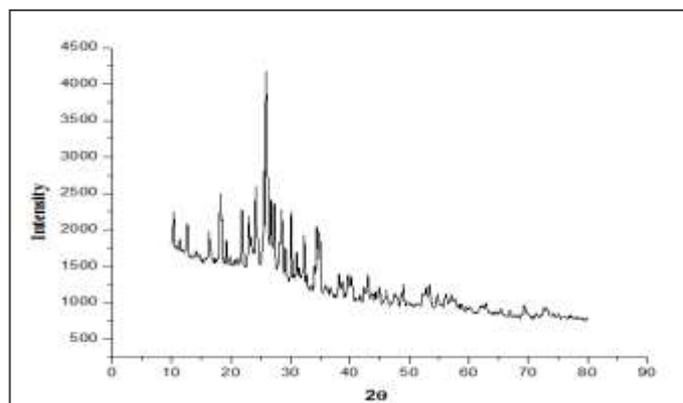
**Fig. 7 XRD spectra of Synthesized Product when pure Graphite used as a Anode**
