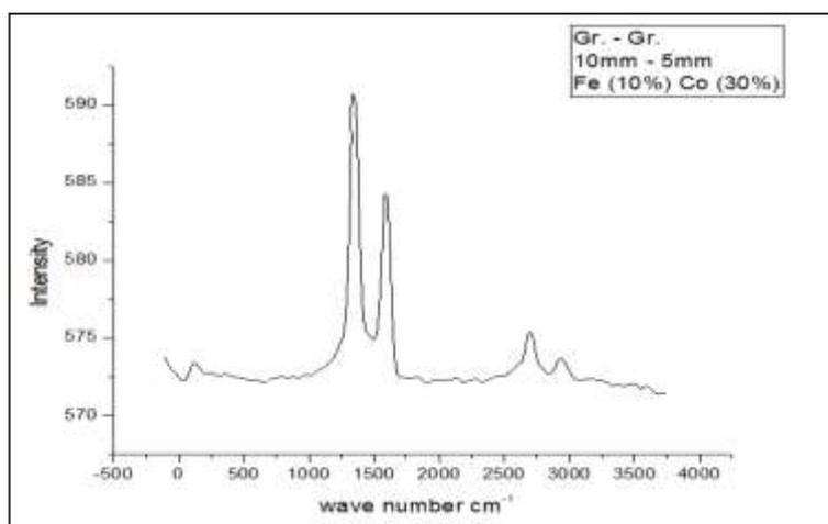
**Fig. 10 Raman analysis of Synthesized Product when doped Graphite used as a Anode**
