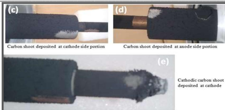
**Fig. 4 Carbon shoot deposited on cathode & Anode.**
