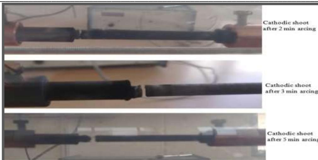
**Fig.6 Cathodic shoot with respect to time interval**
