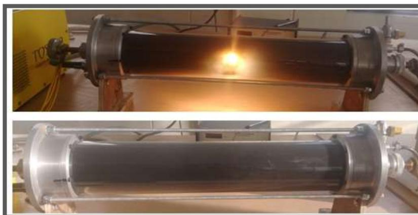
**Fig. 3 Intensity of Arching Plasma when arching with pure graphite rod as anode**
