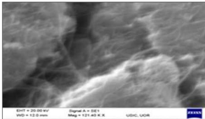
**Fig. 12 SEM image when Fe + Co nano powder mixture doped**
