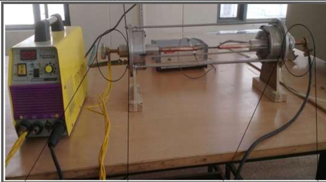
**Fig. 2 Lab setup of electric Arc discharge setup under inert Gas Environment**
