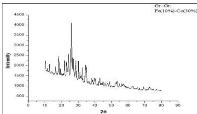
**Fig. 8 XRD Spectra of Synthesized Product when doped Graphite used as a Anode**
