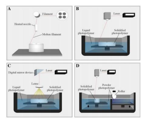
Figure 1: Illustrates the Graphical illustrations of 3DP processes. (A) FDM printer (B) SLA printer (C) DLP printer (D) SLS printer [3]
